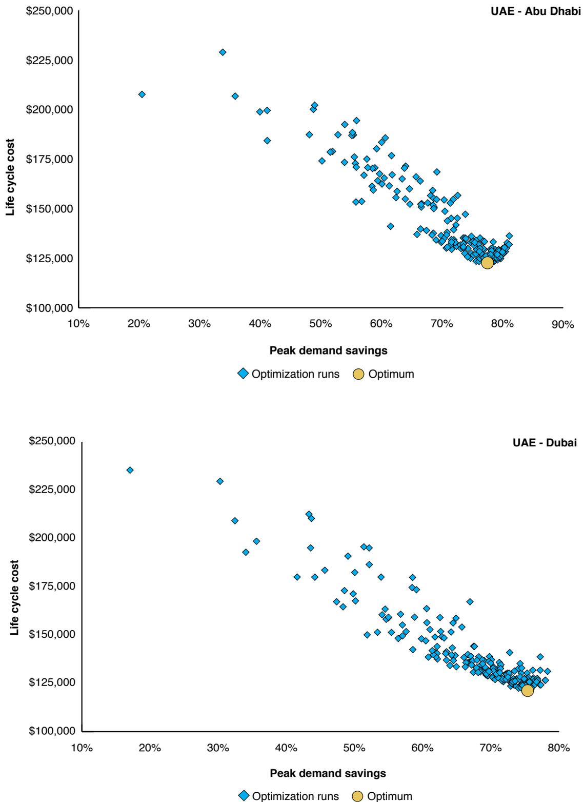
**Figure 13.** Optimization analysis showing peak demand savings against life cycle costs for a villa in (a) Abu Dhabi and (b) Dubai.
